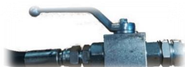
Figure 3. Hydraulic circuit cut-off valve
